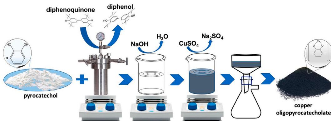
Fig. 1. General scheme for the synthesis of copper oligopyrocatecholate.
